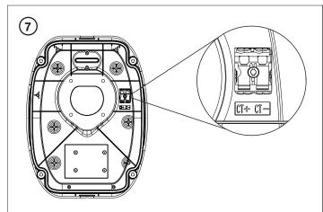
For dynamic load balancing, ensure connections are made in correct polarity to CT+ (Brown) and CT- (Blue) terminals.
