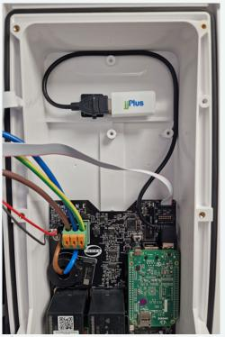
Figure 12: Smart PRO Dongle Placement
