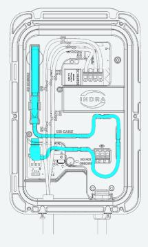
Figure 9: Smart LUX™ Dongle Routing
