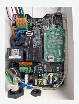
Figure 14: Smart PRO Data Cable Routing
