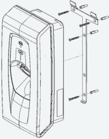
Figure 2: Smart PRO Wall Mounting
