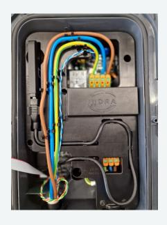
Figure 15: Smart LUX™ 4G Dongle Placement
