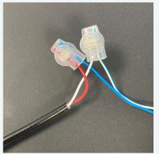
Figure 18: Data Cable Jelly Crimps
