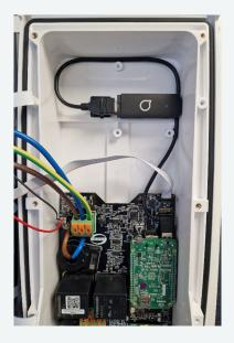
Figure 16: Smart PRO 4G Dongle Placement
