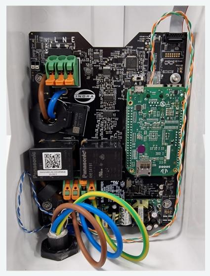
Figure 7: Smart PRO Mains Cable Routing
